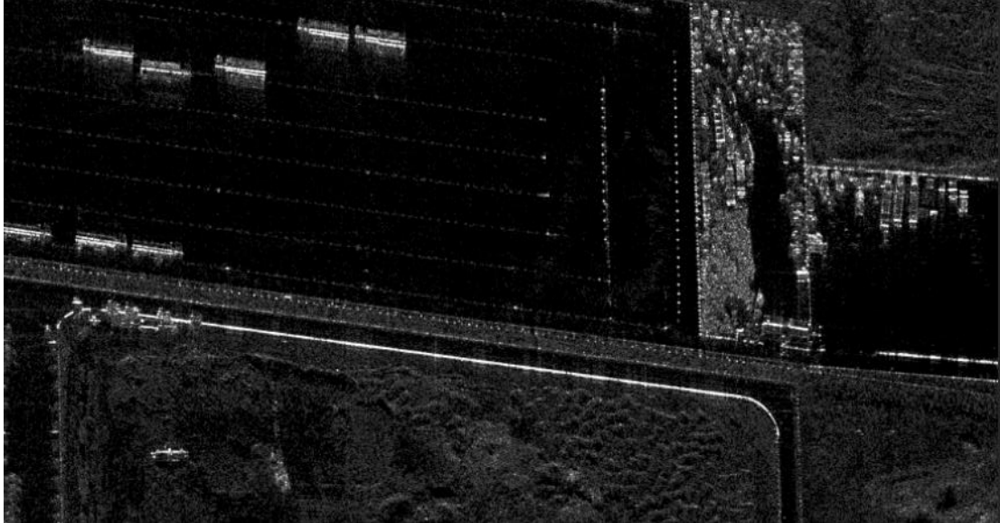
Figure 7 A SAR Image for Car Targets
