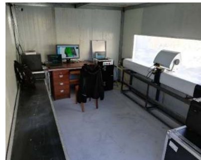
(b) 地基雷达LSA监测系统 (b) Ground-based radar LSA monitoring system
