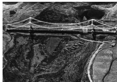
(b) 中科院空天院的机载0.3 m SAR图像 (b) 0.3 m image of AIRI aerial system of Chinese Academy of Sciences
