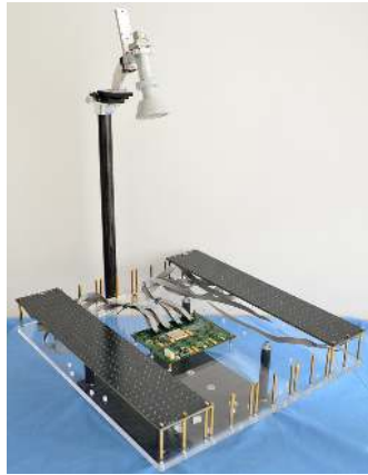
(a) 阵面和FPGA控制板 (a) Array aperture and FPGA control board
