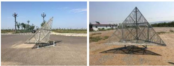
图4 布设于定标场内的角反射器 Fig. 4 Corner reflectors deployed in the calibrating area
